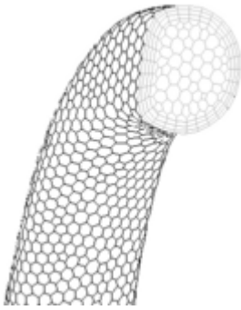
Figure 6.88: The Converted Polyhedral Mesh
