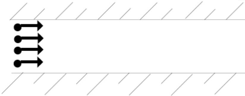
Figure 23.15: Particle Injection Defining an Initial Spray Distribution of the Particle Velocity
