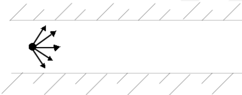
Figure 23.15: Particle Injection Defining an Initial Spray Distribution of the Particle Velocity
